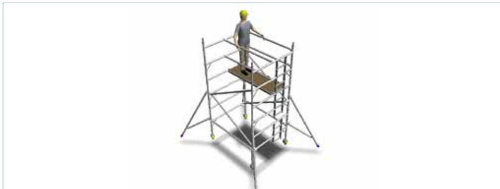
1.26 Clip diagonal braces into position.
