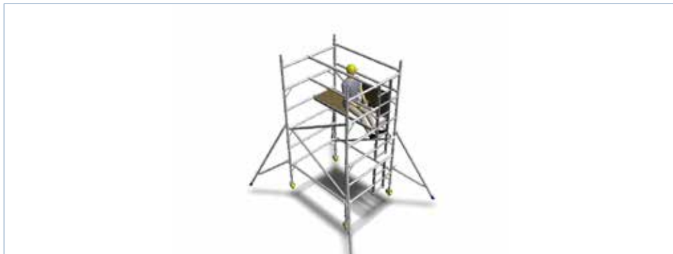
1.26 Clip diagonal braces into position.
